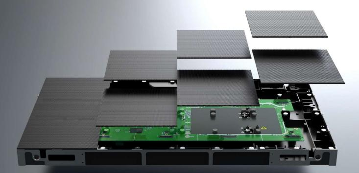
Power supply, receiving card and hub board are integrated on one board, and module connection applies hard connection mode without complex wiring, ensuring stable performance.
